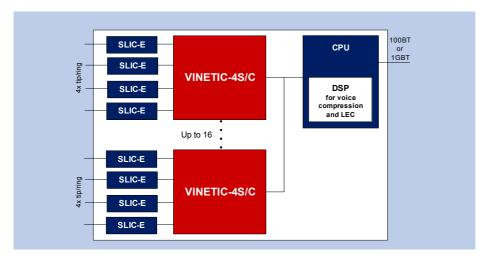
Application Example: VoIP Linecard with integrated Ringing
